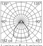
Luminous flux luminaire 2400 lm
