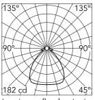
Luminous flux luminaire 2400 lm
