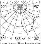
Luminous flux luminaire 816 lm
