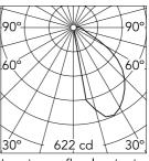
Luminous flux luminaire 800 lm
