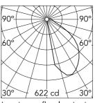
Luminous flux luminaire 800 lm
