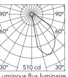
Luminous flux luminaire 656 lm
