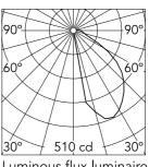
Luminous flux luminaire 656 lm
