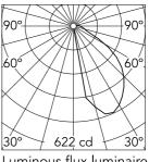
Luminous flux luminaire 800 lm
