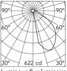
Luminous flux luminaire 800 lm
