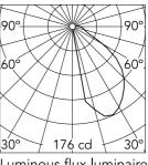
Luminous flux luminaire 210 lm
