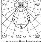
Luminous flux luminaire 744 lm
