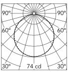
Luminous flux luminaire 200 lm
