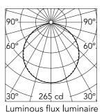
Beam Angle: 111° E(Ix)h(m) D(m) 265 2.89 2 5.79 66 3 29 8.68 4 17 11.57 5 11 14.46
