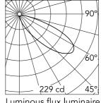
Luminous flux luminaire 479 lm
