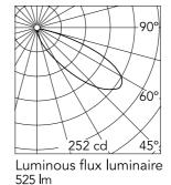
35° Beam Angle: h(m) E(Ix)D(m) 1 252 2.18 2 63 4.36 3 28 6.54 4 16 8.72 5 10 10.90
