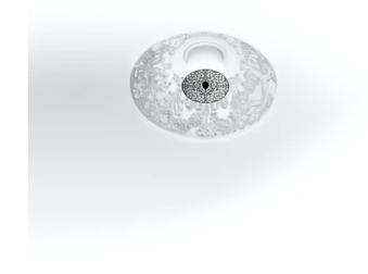
Recessed luminaire providing diffused lighting. Hemispherical, cast plaster diffuser, painted white inside. Plaster diffuser support in die-cast aluminum alloy. Flashed and blown opal glass diffuser. Frieze in photo-etched and mechanically drawn aisi 304 steel.
