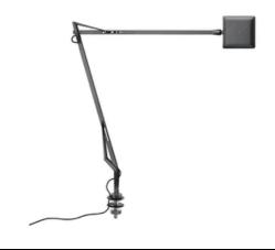
Adjustable table lamp providing direct light. Aluminium painted or chromed body, with die cast head, joints and forks, and extruded arms. Diffuser in photoengraved polycarbonate and aluminate on the perimeter. Edge Lighting technology light source. Optical switch sensor placed on the head that provide 3-step dimming function and color temperature adjustment at 2700K or 3200K. Power cord length 150 cm. Plugin power supply with interchangeable plugs.
