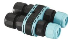
3/4 way terminal block 4 poles IP68 H20 stop. (ø5,5÷12mm cable)
