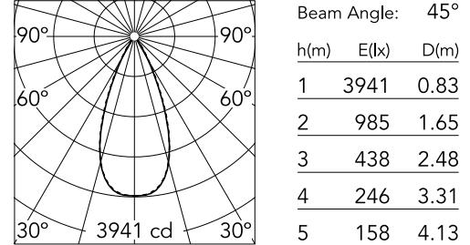
Luminous flux luminaire 2637 lm
