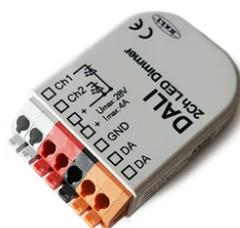
DALI PWM control interface 24Vdc 90W
