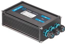
Power supply 24Vdc 20W / 110-240Vdc (15W@110V) IP67 Class II selv. Dimmable DALI
