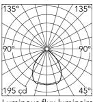
Luminous flux luminaire 4350 lm
