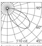
Luminous flux luminaire 212 lm
