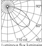
Luminous flux luminaire 212 lm
