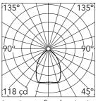
Luminous flux luminaire 4350 lm
