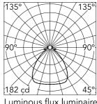
Luminous flux luminaire 2400 lm
