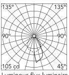
Luminous flux luminaire 92 lm
