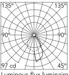
Luminous flux luminaire 85 lm
