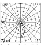
Luminous flux luminaire 55 lm
