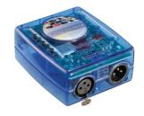
Power supply 24V 10W /110-240V IP20 Class II selv. Non Dimmable RF25747 DMX controller; stand-alone/pc interface.
