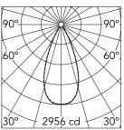
Luminous flux luminaire 1978 lm
