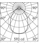
Luminous flux luminaire 1299 lm
