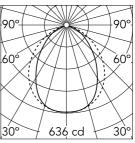
Luminous flux luminaire 1392 lm
