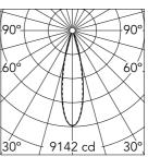
Luminous flux luminaire 2127 lm
