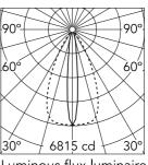
Luminous flux luminaire 1928 lm
