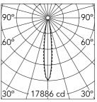
Luminous flux luminaire 2189 lm
