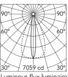
Luminous flux luminaire 1997 lm
