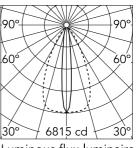
Luminous flux luminaire 1928 lm
