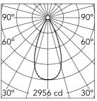
Luminous flux luminaire 1978 lm
