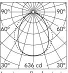
Luminous flux luminaire 1392 lm
