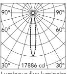
Luminous flux luminaire 2189 lm
