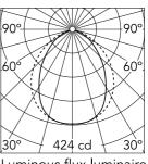
Luminous flux luminaire 928 lm
