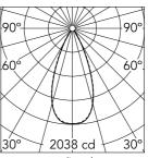
Luminous flux luminaire 1364 lm
