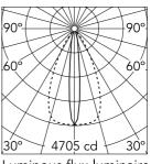
Luminous flux luminaire 1331 lm
