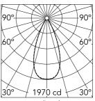
Luminous flux luminaire 1318 lm
