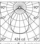
Luminous flux luminaire 928 lm
