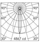
Luminous flux luminaire 1377 lm
