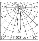
Luminous flux luminaire 1411 lm
