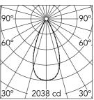
Luminous flux luminaire 1364 lm
