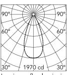
Luminous flux luminaire 1318 lm
